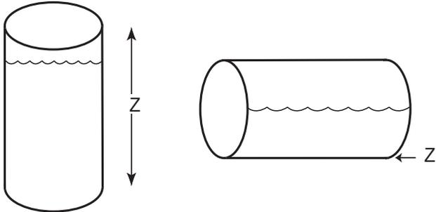
For most vessels, the zero reference point (Z) may be designated as any height in the vessel.
