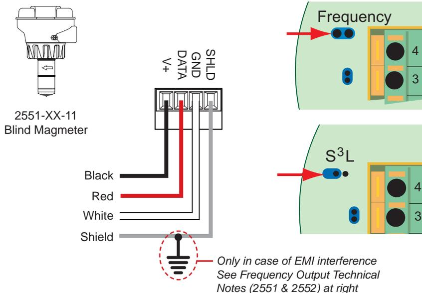
**Input Wiring for 2551 and 2552 sensors**
