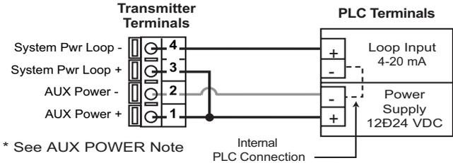
Example: Two transmitters connected to PLC/Recorder with separate power supply
