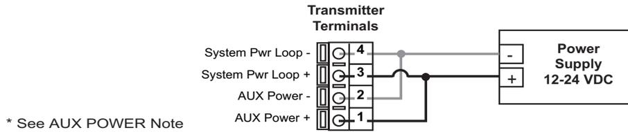
Connection to a PLC/Recorder, separate supply
