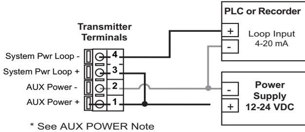
Connection to a PLC with built-in power supply
