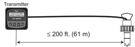
Maximum cable length is 1000 ft. for 2536/8512-XX, 2540/2541, vortex, and any open-collector flow signal.
