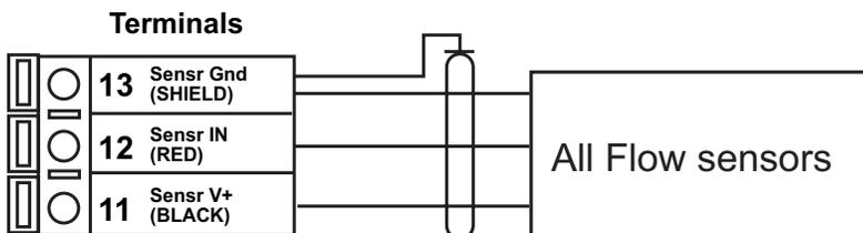
Maximum cable length is 200 ft. for 515/8510-XX, 525 , 2517 and any sinusoidal flow signal.
