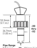
0.5 to 4 in. -X0 = 104mm (4.1 in) 5 to 8 in. -X1 = 137mm (5.4 in.) 10 in. and up -X2 = 213mm (8.4 in.)
